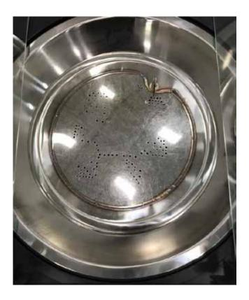
Oxidization does not affect the performance of the burner, and the weld will be covered by fire glass, so this will not be visible.
