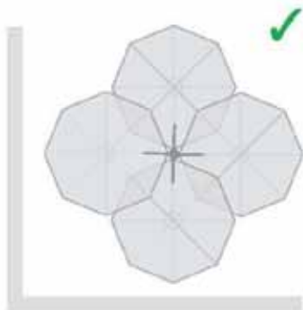
GOOD RULE OF THUMB WHEN INSTALLING AN UMBRELLA WITH FULL 360°, MEASURE FOR CANOPY ON EACH SIDE
